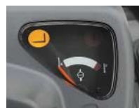
Lifting interlock lamp on the meter panel
