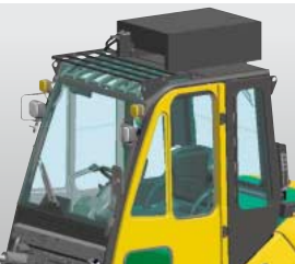
Steel cabin with cooler
