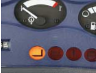
Lifting interlock lamp on the control panel
